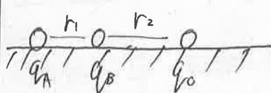
$$k \frac{q_B q_C}{r^2} = k \frac{q_A q_B}{r_2^2} = k \frac{q_A q_C}{(r+r_2)^2}$$
