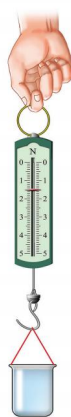
(c) 接水后杯子与水总重 G'_{\text{杯}} = \underline{\quad} N, 被物体排开水的重力 G_{\text{排}} = G'_{\text{杯}} - G_{\text{杯}} = \underline{\quad} N
